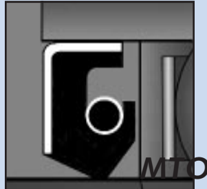
Spring Loaded "V" Seal
