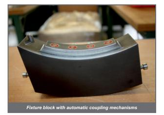
Before use of the AKM the experts in Chemnitz laboriously generated the coupling function using an additional moved axis with a stroke of 5 mm. Alternatively they had thought about a multi-channel rotating bush. However, the realisation of this idea was somewhat problematic, firstly, due to the high rotational speed and secondly because the required installation space was not available. Support with the AKM functions reliably according to their test since 2014.
